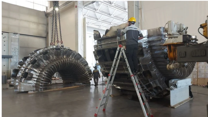
SPARC vacuum vessel ready for shipment
